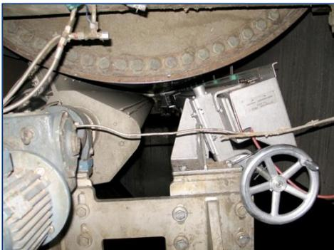
**EV ReDoc®** is a continuous reconditioning system for paper machine cylinder and roll surfaces. EV ReDoc -system eliminates dirt like stickies, fibres and coating colour from cylinder surfaces by using steel brushes.
