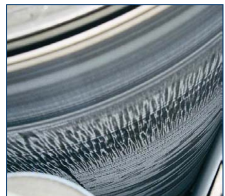
Fibers, starch and chemicals have created an isolating layer onto cylinder surface.
